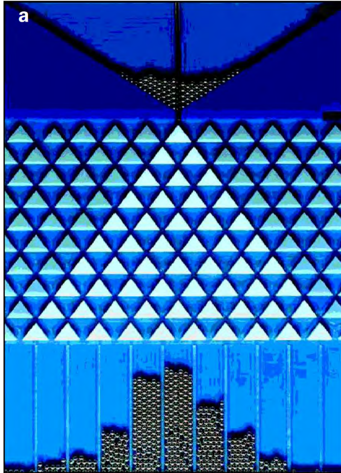
Figure 2. Physical models demonstrating the genesis of normal and log-normal distributions. Particles fall from a funnel onto tips of triangles, where they are deviated to the left or to the right with equal probability (0.5) and finally fall into receptacles. The medians of the distributions remain below the entry points of the particles. If the tip of a triangle is at distance x from the left edge of the board, triangle tips to the right and to the left below it are placed at x + c and x - c for the normal distribution (panel a), and x \cdot c' and x / c' for the log-normal (panel b, patent pending), c and c' being constants. The distributions are generated by many small random effects (according to the central limit theorem) that are additive for the normal distribution and multiplicative for the log-normal. We therefore suggest the alternative name multiplicative normal distribution for the latter.
