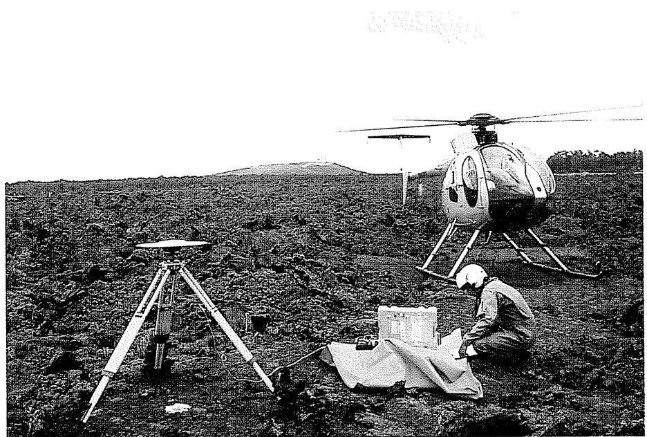
Fig. 1. David Okita deploys a GPS receiver near Pu'u O'o, Hawaii—Kilauea volcano's most active vent. Scientists from Stanford University and the U.S. Geological Survey, with equipment and logistical support from UNAVCO, have taken GPS measurements on Kilauea since 1987. The goal of the experiment is to better understand the kinematics and mechanics of the deformation associated with Hawaiian volcanism. (Photo: Peter Cervelli).
