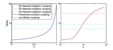
FIG. 4. Equilibration time versus perturbation from meanfield coupling. Shown is the simulation time required for the system to evolve from 10% to 90% of the way between its initial condition and the thermalized (zero net magnetization) steady-state. Left panel: piecewise-constant coupling (8); right panel: von Mises coupling (9). Also shown, for reference, is the equilibration time for 2, 3, and 4-dimensional nearestneighbor coupling (higher dimensions equilibrate faster).
