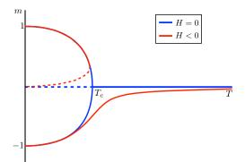
FIG. 2. Steady-state magnetization versus temperature for homogeneous system, Eq. (6). For H = 0 there is a supercritical pitchfork bifurcation, while for  $H \neq 0$ , the bifurcation becomes imperfect. Solid lines indicate stable solution branches, dashed unstable.
