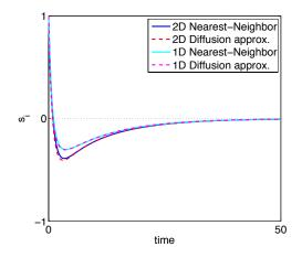
FIG. 5. Perturbed spin versus time. To test the approximation to the dynamics in Eq. (10), the system was initialized with a single spin  $s_i = +1$  while the rest of the system was aligned at -1. The time evolution of this misaligned spin is shown for 1D and 2D nearest-neighbor systems together with the diffusive approximation. (The curves in 3D are similar and are omitted for clarity.)
