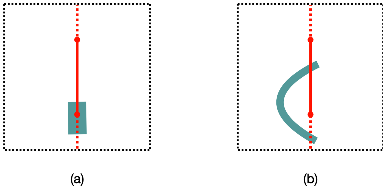
Figure 2.4: Two different clusters can give a corner contribution. a). A cluster directly touching a corner is encountered by both line segments. b). A “rainbow-shaped” cluster also contributes since it encounters both half-line segments even without touching the corner. Such clusters are only expected to occur at criticality.
