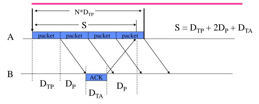
• We want to choose N large enough to allow continuous transmission while waiting for an ACK for the first packet of the window,
