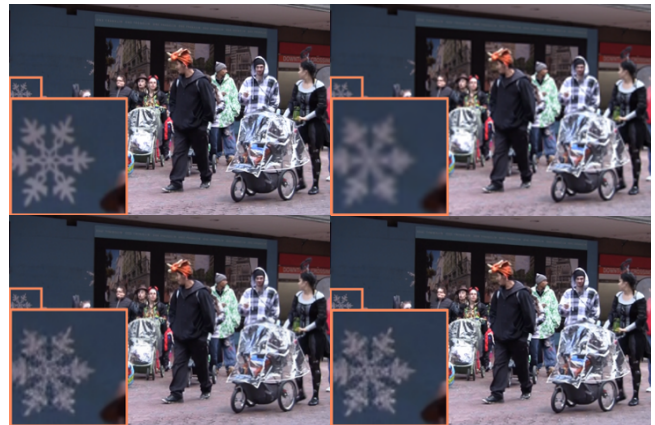
Fig. 5: Qualitative comparison of VSRResFeatGAN [12] (2nd row, left) vs. Spatially Adaptive VSRGAN (2nd row, right) on scale factor 3, with ground Truth (1st row, left) and input low-resolution (1st row, right).
