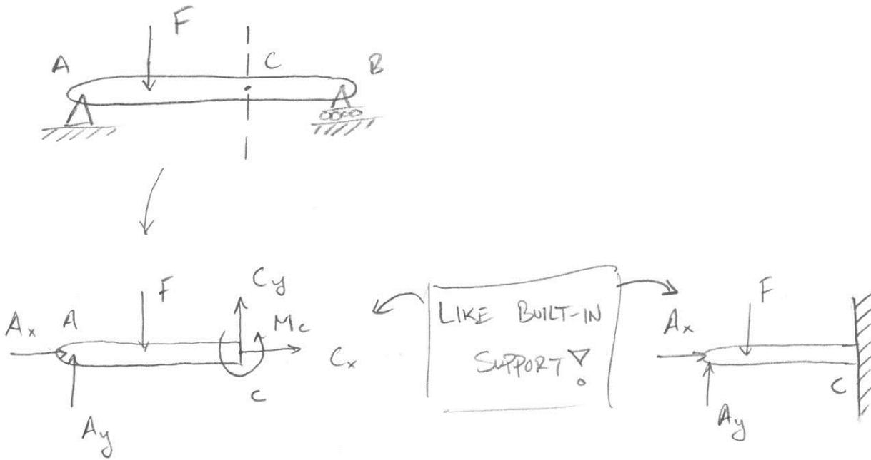
The internal forces change depending on the location of the cut! In this case the moment ( $M_C$ ) changes continuously. You will do more with this in CIV\_ENV 216 (*Mechanics of Materials*).
