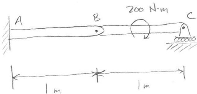
Determine the reactions at *A* and *C* and the internal forces at *B*.
